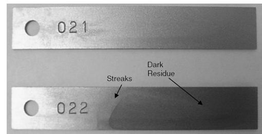
Fig. 13. Grey cast iron corrosion coupons after exposure to 80% and 20% biofuel for 10 months (7342 h). 021 = Grey cast iron stored in 20% biofuel and 022 = grey cast iron stored in 80% biofuel.
